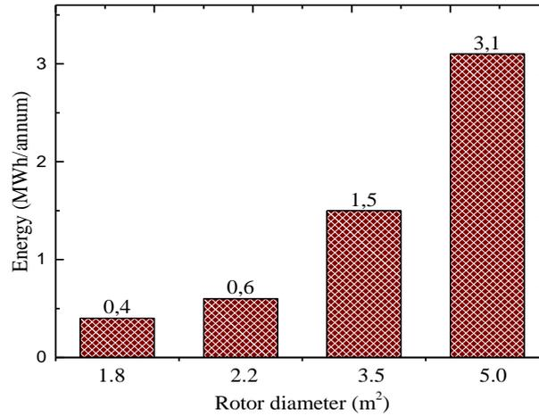
Fig. 5. Wind energy conversion by Poldaw wind pumps at 10 m hub height ( $v_m = 4.22$  m/s) in the Keta municipality.
