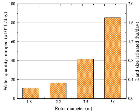
Fig. 4. Performance of Poldaw wind pumps at  $v_m = 4.22$  showing estimated water quantities and farm size it could irrigate in Keta.
