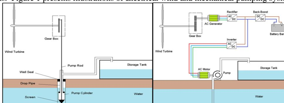
Fig. 1. Schematic representations of Electrical Wind (left) and Mechanical Wind (right) pumping systems (Achour & Kesraoui, 2021).
