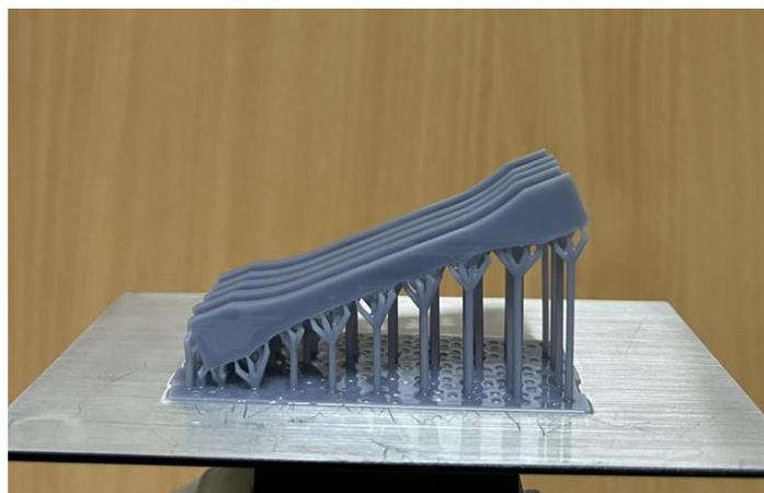
Fig. 15. SLA 3D printed resin samples angles 22.5 degree and side orientations.
