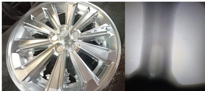
Fig. 2 Hot spot in rims
