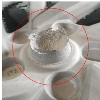
Fig. 8 Porosity in hub area
