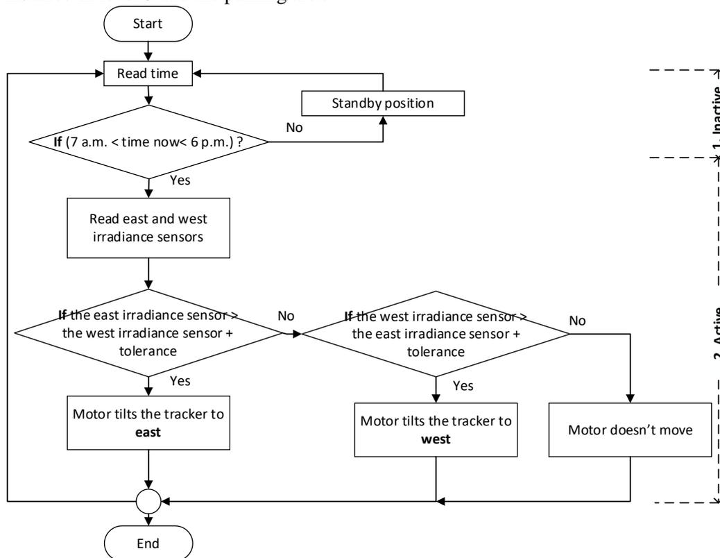
Fig. 3. Flowchart of closed-loop control of single-axis solar tracker
