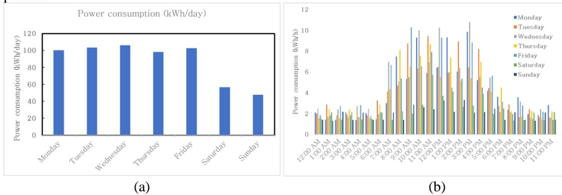
Fig. 4. Load profile of electricity consumption at level 4 a) daily and b) hourly
