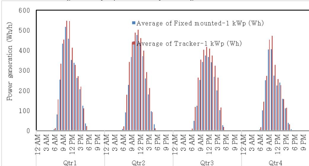
Fig. 12. Electricity generation from fixed mounted and tracked mounted PV panels quarterly over
