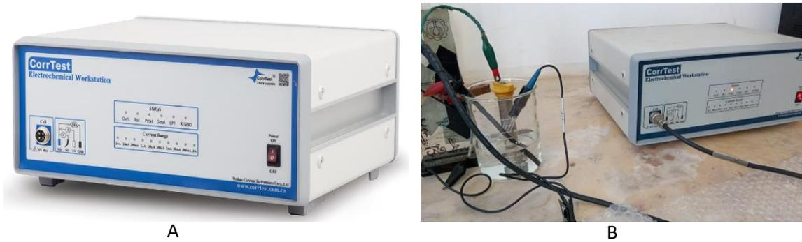
Fig. 5. Potentiodynamic testing process: a) equipment; b) equipment circuit
