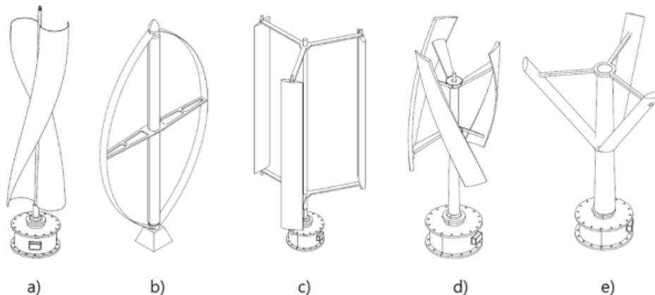
Fig. 1. Graphical representation of various types of Vertical Axis Wind Turbines (VAWT): (a) Savonius, (b)  $\phi$ -Darrieus, (c) H-rotor Darrieus, (d) Helical bladed, (e) V-shaped
