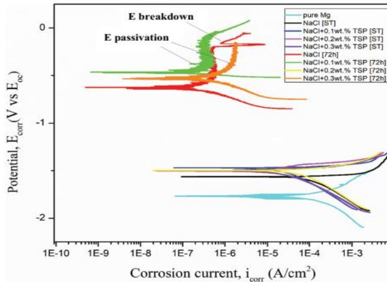
Fig. 4. Tafel curves for Mg-5Sn-0.2Ca-0.2Mn at various immersion periods across different electrolyte concentrations.
