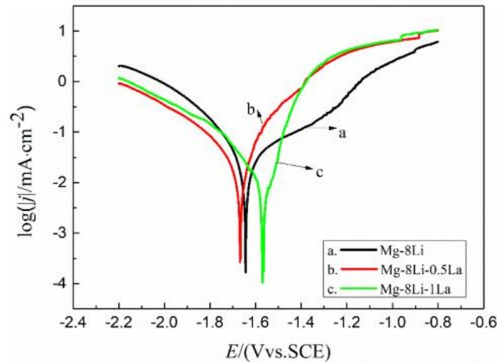
Fig. 3. Potentiodynamic polarization curves for the electrodes: (a) Mg-8Li, (b) Mg-8Li-0.5La, and (c) Mg-8Li-1La
