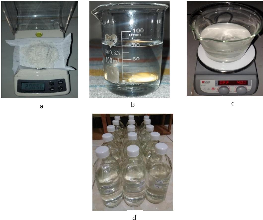
Fig. 4. Steps for making salt solution: a) weighing salt; b) measuring the volume of water; c) stirring; d) salt solution ready for use
