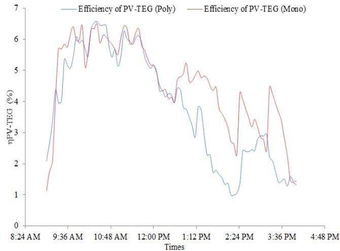
Fig. 7. The efficiency of hybrid PV-TEG; (a) PV Polycrystalline, (b) PV Monocrystalline
