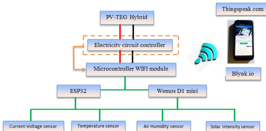
Fig. 3. Flowchart of the Sensor System in PV-TEG Hybrid
