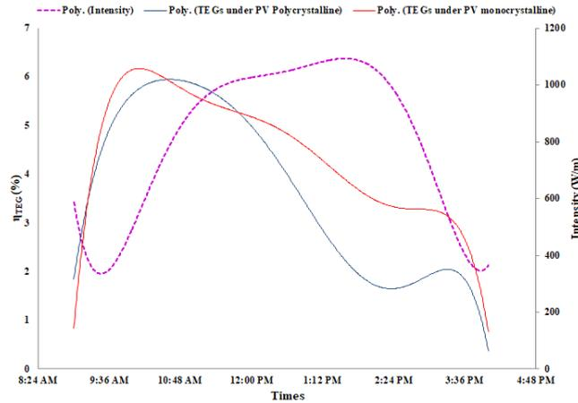
Fig. 5. Effect of Solar Intensity on the Performance of PV-Hybridized TEG Modules
