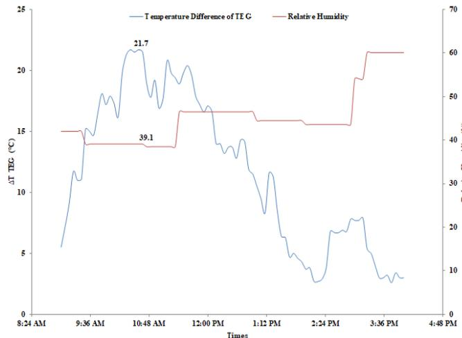
Fig. 6. Effect of Air Humidity on Temperature Difference in PV-Hybridized TEG
