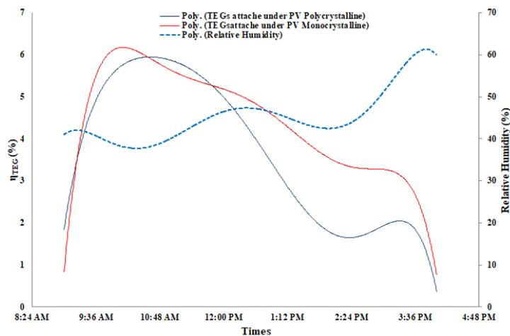
Fig. 4. Effect of Air Humidity on the Performance of TEG Hybridized with PV
