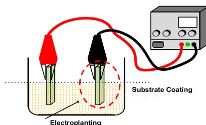
Fig. 1. Element of electroplating and process of electroplating
