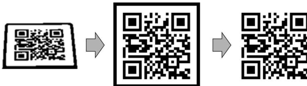
Fig. 3. Normalization of the pattern and matching template
