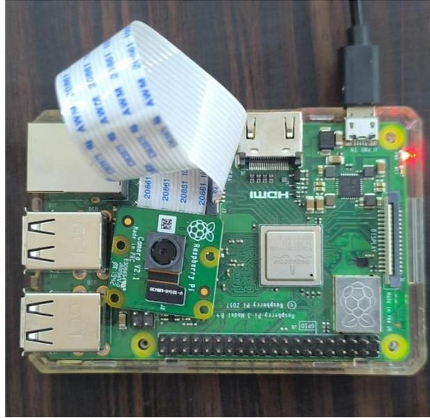
Fig. 5. The utilised Raspberry Pi-3 with the compatible camera
