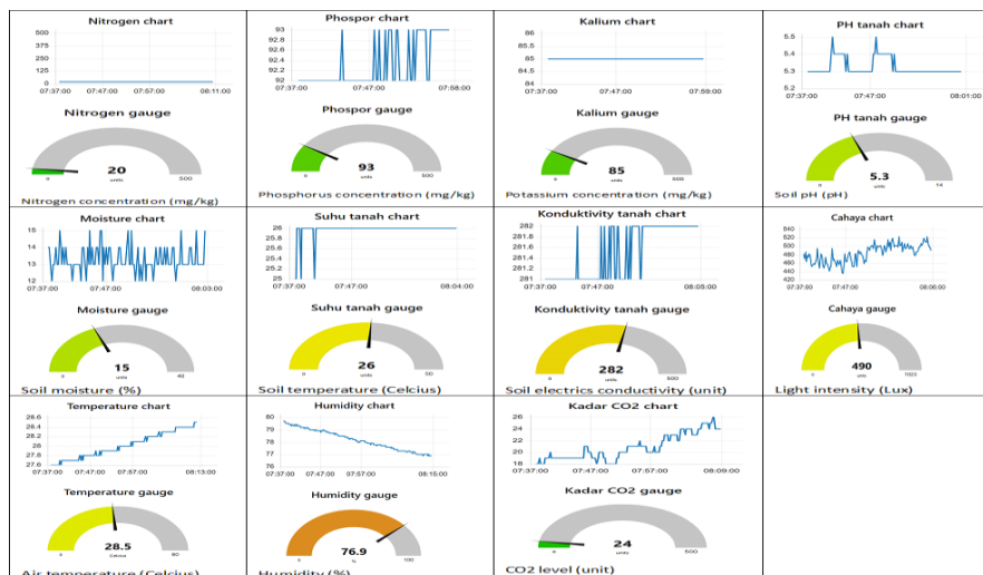
Fig 6. NodeRed Dashboard: Chart and Gauge Output
