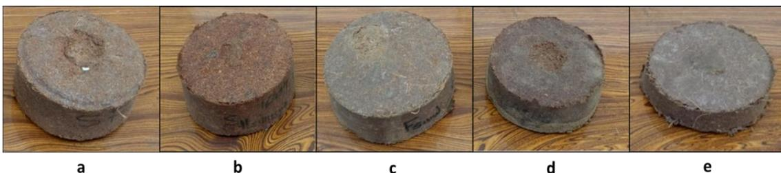
Fig 1. Test specimens, (a) mixture of fine grade sawdust and coconut fiber, (b) fine grade sawdust; (c) mixture of coconut fiber, fine grade sawdust and expansive clay, (d) a mixture of fine grade sawdust and expansive clay. (e) mixture of coconut fiber and expansive clay
