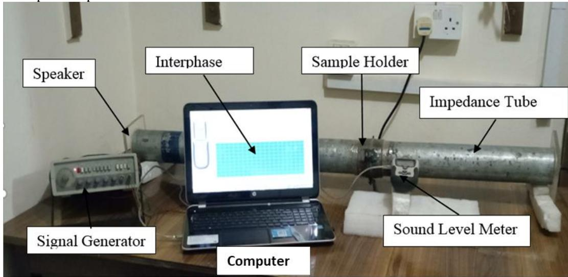
Fig. 2. Experimental setup for sound reduction measurement
