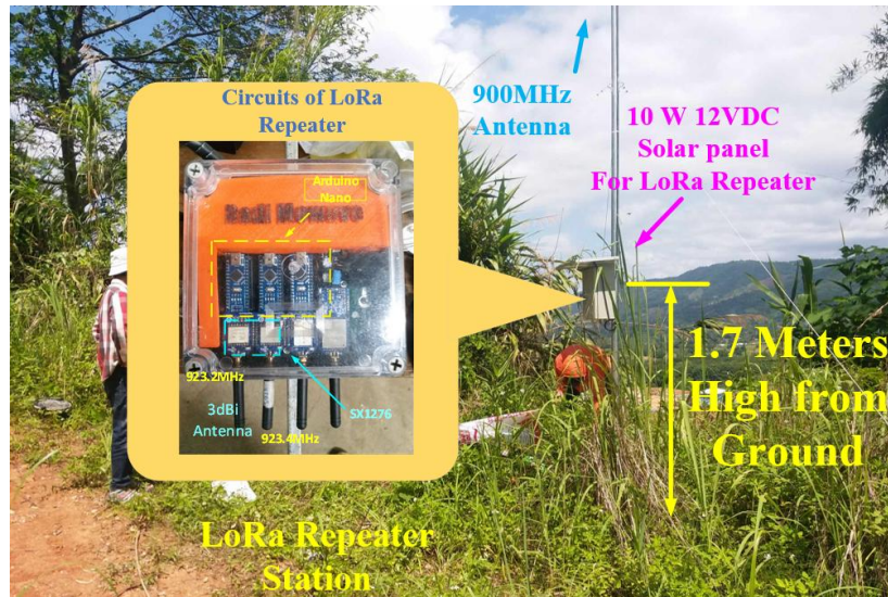
Fig. 8. The installation site of the LoRa repeater is shown.
