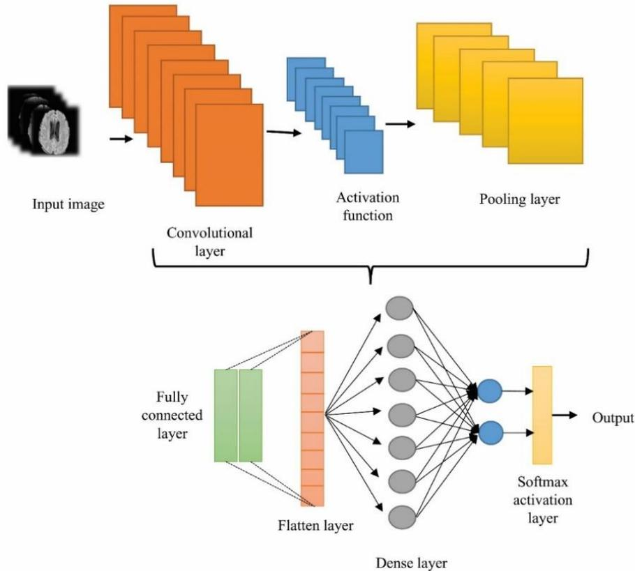
Fig. 3. Proposed Architecture of CNN based VGG-16
