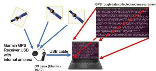
Fig. 1. Measurement and GPS data acquisition system
